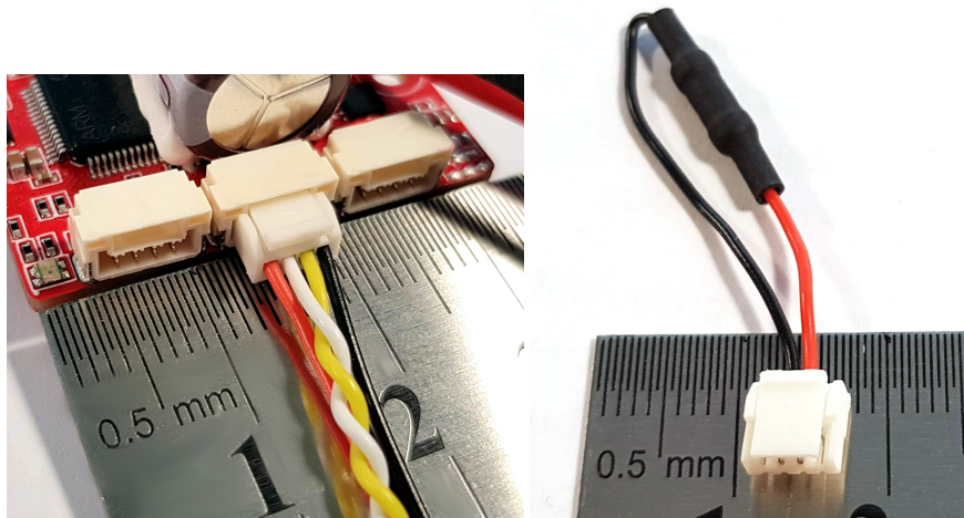
Right-angle connector with a twisted pair cable connected; a 120Ω termination plug.
