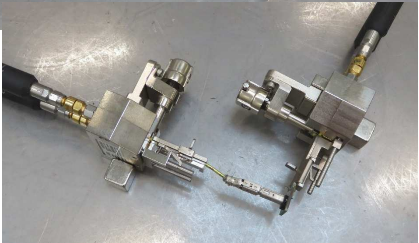
Test setup with prototypes (not the final contact design and serial plastic material) and HARTING BCCTF-40GHz test fixture and network analyzer
